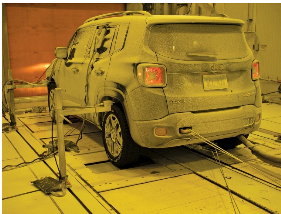
A 2015 Jeep Renegade Trailhawk grows an icy coat inside CTC's newly revamped climatic test chamber equipped with a 4x4 dynamometer.
