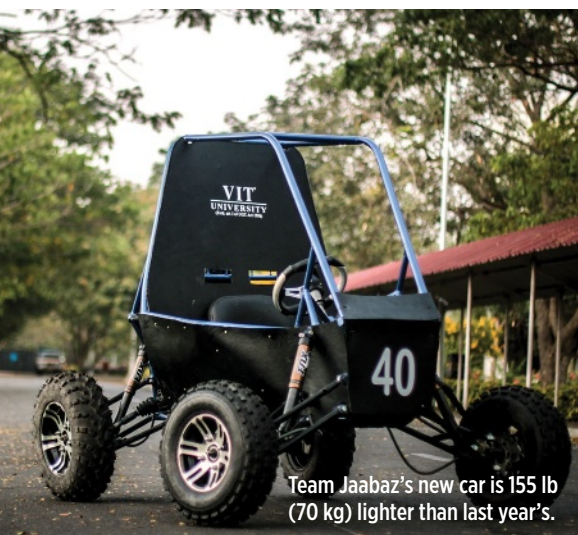
The front upright was completely redesigned and produced a weight reduction of 40% and a cost reduction of 75% compared to the previous unit.
