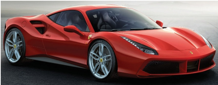
The base bleed air intakes on the car's flanks are divided by a flap with flow over the upper section directed to the engine and the lower flow to the intercoolers.
