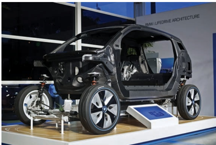
The BMW i3 electric vehicle incorporates many lightweight components, including a carbon-fiber body that is glued and bolted onto an aluminum chassis.
