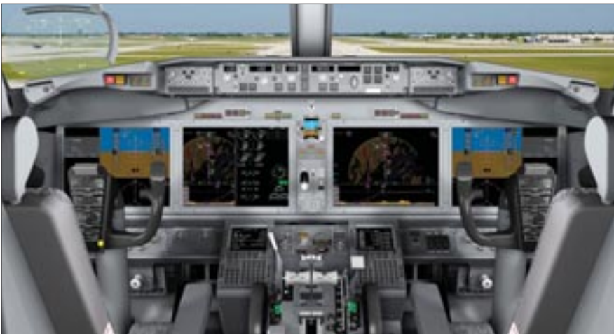
Artist's rendering of the 737 MAX flight deck with four new large-format displays.
