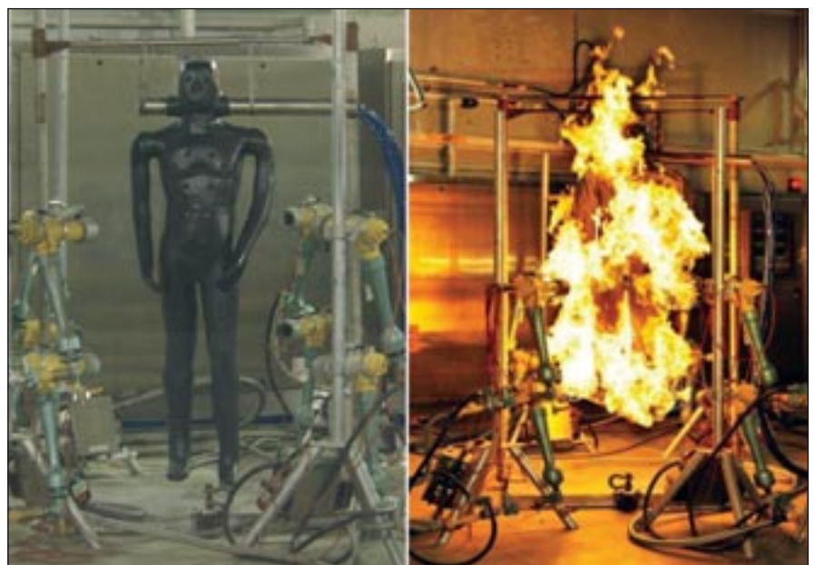
Figure 1. The flash flame test conducted on the thermal test manikin.
