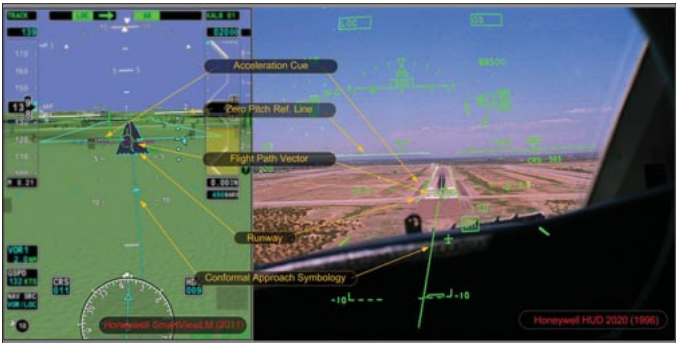
Figure 2. The integration between the Honeywell SVLM with FPV and runway approach symbology created in 2011 (left) based on Honeywell HUD2020 (right) created in 1996 providing the same functionality is shown above. LEFT: This screen capture is of an SVLM prototype installed in the company's Gulfstream 450. The approach shown was an ILS to runway 01 at Albany International Airport New York (KALB). RIGHT: This photograph was taken through the HUD combiner of the prototype HUD2020 installed in a Cessna Citation III. This approach was an ILS to runway 30C at Williams Gateway Airport, Phoenix Arizona (KIWA).
