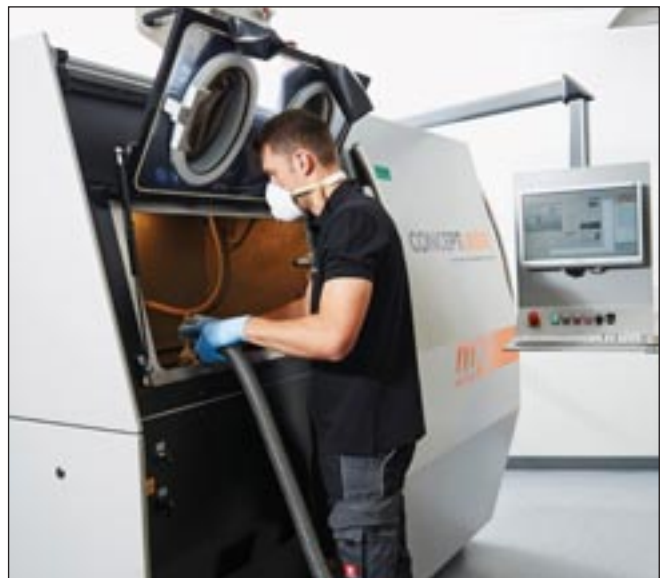
Toolcraft uses laser melting machines from Concept Laser that offer a workspace of 250 x 250 x 280 mm in the x, y, and z directions.
