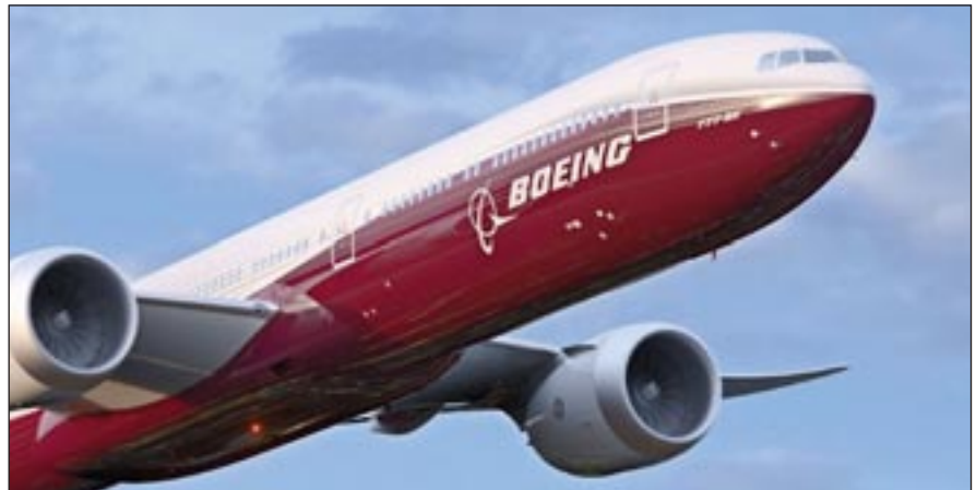
The new 777X will build on the 777 and will include new engines, an all-new composite wing and will leverage technologies from the 787 Dreamliner.
