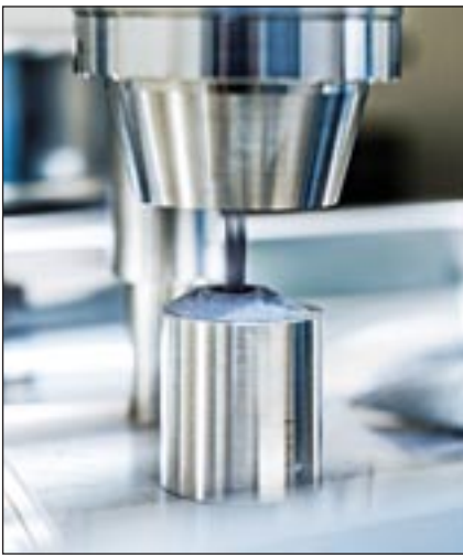
Scalmalloy from Airbus APWorks is a corrosion-resistant material with the specific strength of titanium at a simultaneously high ductility. It is more than twice as strong as the aluminum-silicon powder currently in use.
