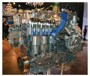
The first F-Pace vehicles to come to the U.S. will be powered by Jaguar's 2.0-L Ingenium turbodiesel four-cylinder engine.
