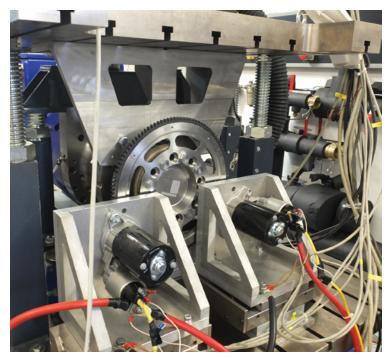
AVL developed a unique test stand for testing start/stop motors, reflecting some of the challenges and opportunities in today's electrified powertrains.
