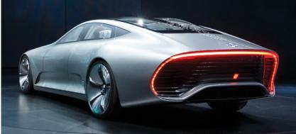
Aerodynamic optimizations for the Mercedes concept include windows that fit flush on the outside, a blue LED touchpad instead of door handles, and lowering of the chassis, resulting in a ground clearance of 100 mm (3.9 in).
