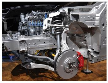
The F-Pace is more than 80% aluminum by weight even using aluminum for parts like suspension castings and the B-pillar.
