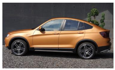
Clemson University's Deep Orange project car relies on Dow Automotive Systems resins for its weight-saving resin transfer molding carbon-fiber bodywork.
