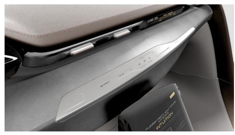
Intuition incorporates a soft aluminum surface called DecoControl Alu, a monitoring and decorative zone set along the lower edge of the IP. Capacitive switches are integrated into the surface. Also note the "invisible" black screen located on the passenger side, shown here lit up in active mode.
