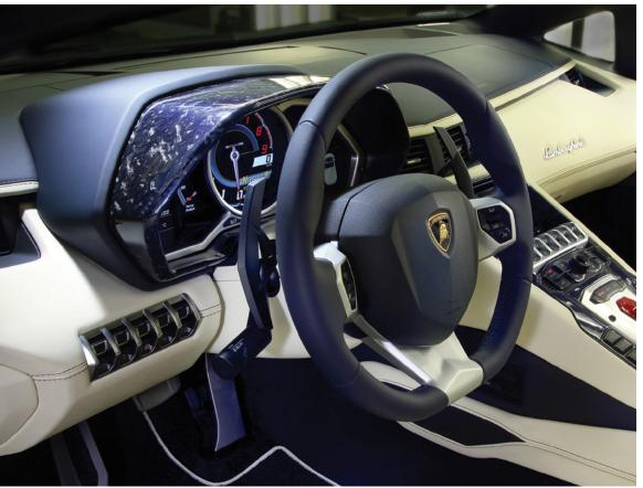
Lamborghini's forged composite technology is on display on this Aventador's instrument surround and is valued for its combination of light weight and unique appearance.
