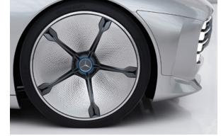
Active wheel rims on Concept IAA change their cupping from 50 mm (2.0 in) to zero—from five-spoke to flat-disc wheels.
