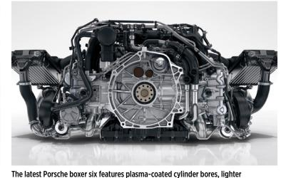
crankcases, an engineered-plastic oil pan, and direct injection that operates at
