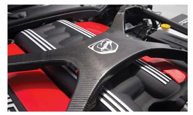
The Dodge Viper's shock tower brace is stronger and lighter thanks to its carbonfiber construction.
