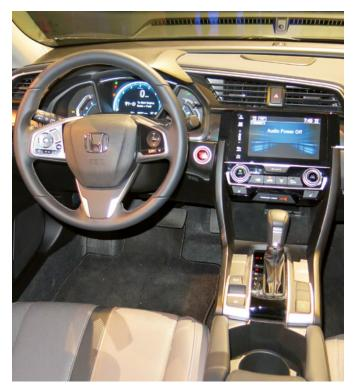
2016 Civic cockpit has improved ergonomics. Driver's H-point is 20 mm lower than previous model, with lower floor, IP, and engine.
