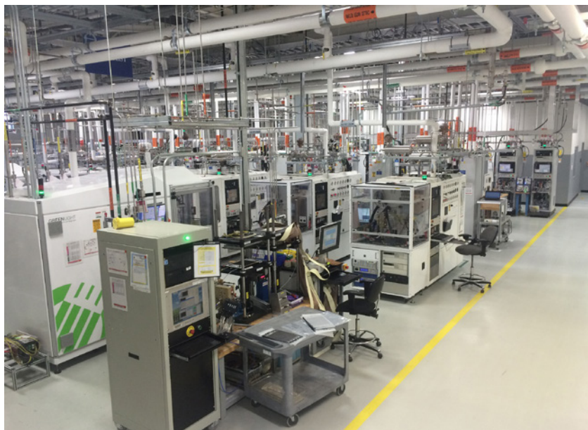
GM's hydrogen fuel cell lab in Pontiac, MI, builds and tests the next generation of fuel cell technology—from single cells to full vehicle sized fuel-cell systems.
