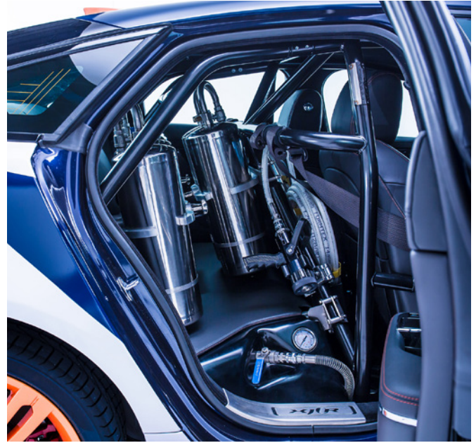
Supercharged Jaguar XJR converted to rapid response fire engine for the Bloodhound Project.
