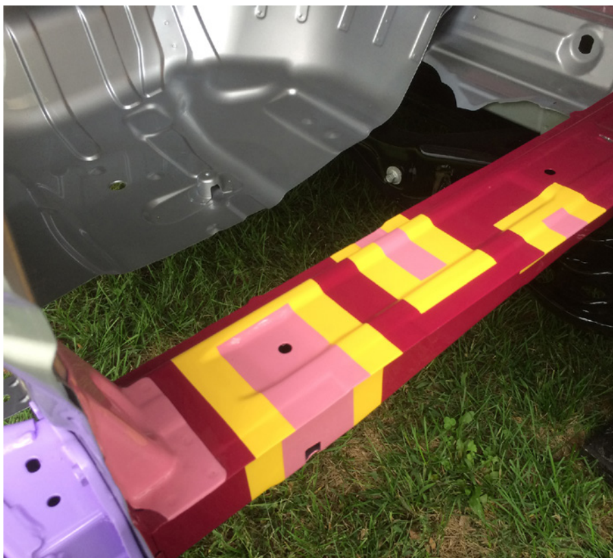
An in-die soft zone on the 2016 Civic’s rear frame rail varies from about 590-MPa advanced high-strength steel (pink) to 1500-MPa press-hardened steel (deep purple). The yellow depicts the transition zone between the two grades. (Ryan Gehm)
