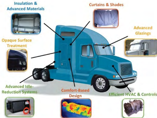
Technologies evaluated in the NREL climate-controlled sleeper program. Advanced glazings were used for reference only.
