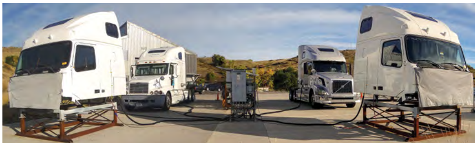
Test bucks and sleeper cabs were evaluated at NREL’s Golden, CO facility. Electrical use was monitored from a 120-V AC source for testing convenience.
