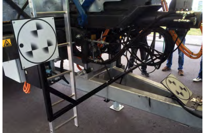
For automatic hitching, currently there are three target shields mounted on the trailer to help guide the system. In the future, the system could use sensor fusion that combines an optical camera and a laser system to eliminate the need for shields. (Photo by Ryan Gehm)
