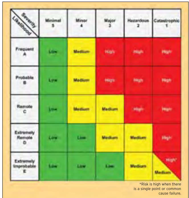
Figure 3. FAA Risk Matrix. Likelihood ranges from an event that is likely to happen once a week (A) to an event that is likely to happen less than once in 30 years (E). Severity ranges from minimal (5) through increasing levels of loss of control (4 to 2) to actual harm (1).
