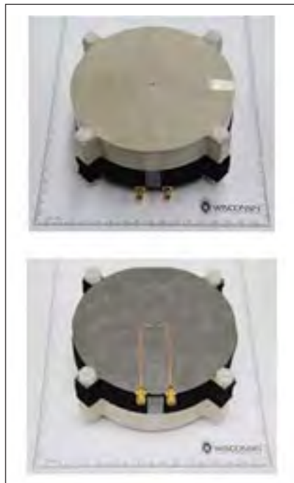
Figure 4. The miniaturized, ground-plane-backed, circularly polarized UWB antenna.
