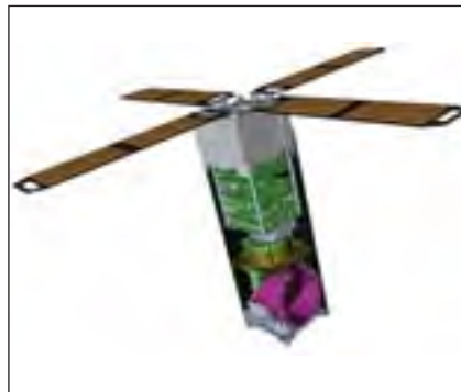
The NanoRacks-MicroMAS nanosatellite with radiometer payload rendering. (MIT Lincoln Laboratory)
