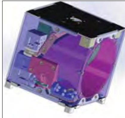
Rendering of a 118-GHz microwave radiometer from the NanoRacks-MicoMAS nanosatellite. (MIT Lincoln Laboratory)
