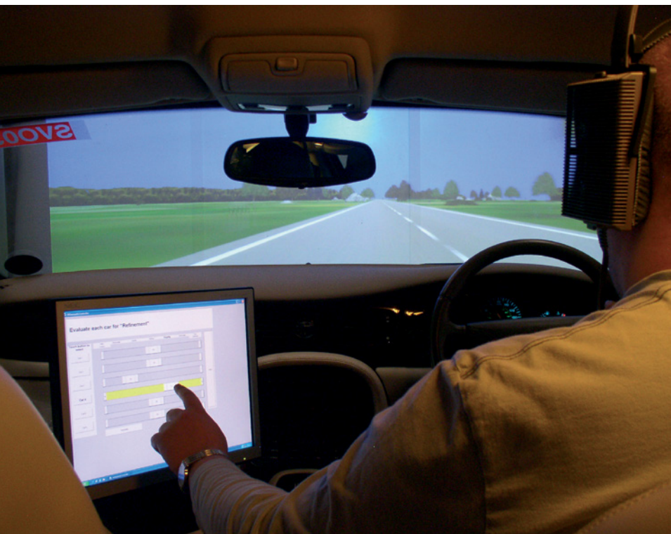
A view "behind the wheel" of Altair Engineering's pioneering full-vehicle NVH simulator.
