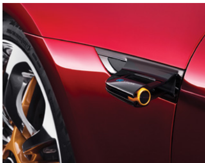
Revealed at the 2017 Geneva Motor Show: Mercedes-AMG GT Concept with rearview cameras instead of door mirrors.
