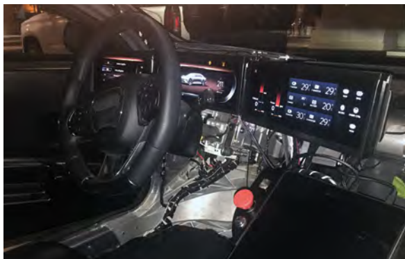
Air prototype's interior: large, vivid data screens and some necessary components borrowed from more prosaic production models (Image: Bill Visnic).
