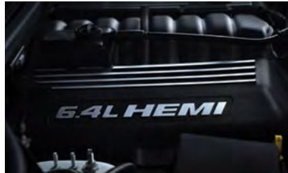
The 6.4-L iron-block OHV V8 generates 475 hp from a 10.9:1 compression ratio. (Image: FCA)
