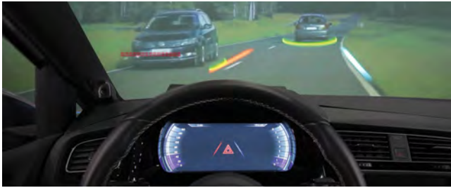
A halo around an oncoming car and other graphic overlays are shown on the AR HUD in Visteon's VW Golf demo vehicle, which also has an exterior forward-facing camera and two driver-facing cameras.
