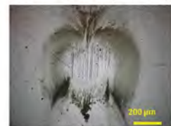
Argonne's Catalyst Coating Tested Neat Oil (PAO-10)
