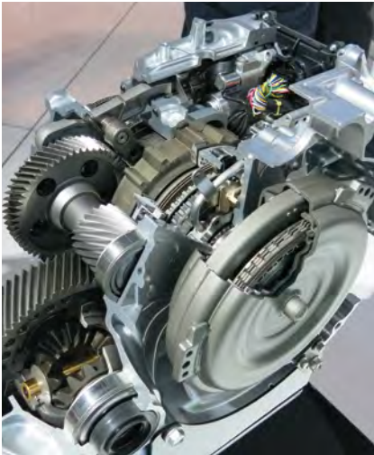
The 10-speed's torque converter is an entirely new design aimed at optimally collaborating with the engine's cylinder deactivation and stop-start systems. (Lindsay Brooke photo)
