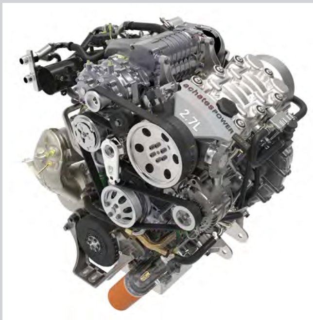
The new 2.7-L three-cylinder OP is engineered for both gasoline and diesel fuels. Note cylinder axis slanted slightly for packaging, supercharger at top of image, and close-coupled catalyst at left center.
