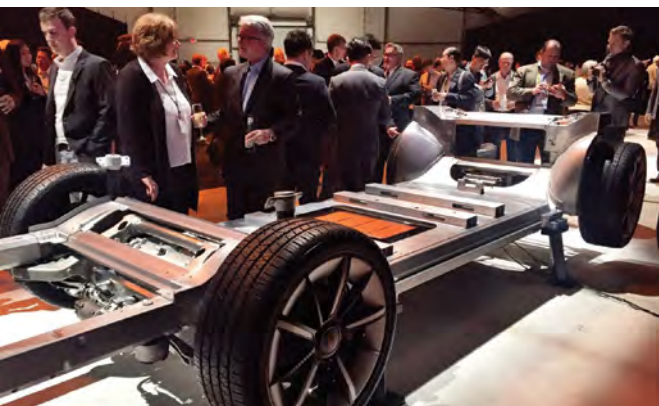
The FF 91 is built on the company's Variable Platform Architecture (VPA), a flexible powertrain and monocoque structure with the batteries under floor. (Kevin Jost image)
