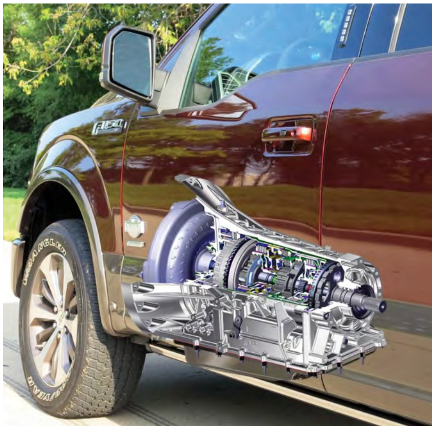
Besides the F-Series application, the new 10R is also available in the 2018 Ford Mustang. (F-150 photo by Lindsay Brooke, 10R courtesy Ford).
