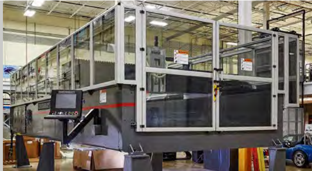
The Department of Energy's Manufacturing Demonstration Facility at ORNL is now home to the world's largest polymer 3D printer. The new BAAM (Big Area Additive Manufacturing) machine is another result of ORNL's yearlong collaboration with Cincinnati Inc.
