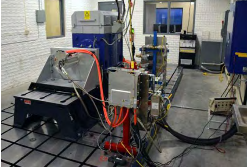
Printed Cobra traction motor installed in ORNL component test cell in the NTRC loop laboratory.
