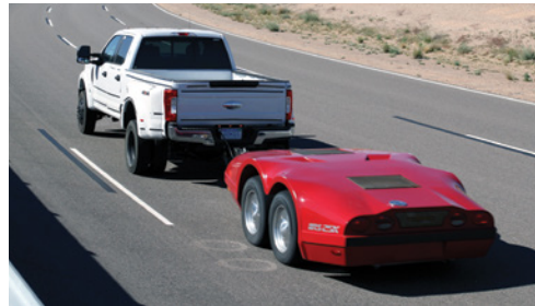
2017 Super Duty prototype with new Taylor RSL-25K dyno sled replicates the Davis Dam climb at Ford's Arizona P.G.
