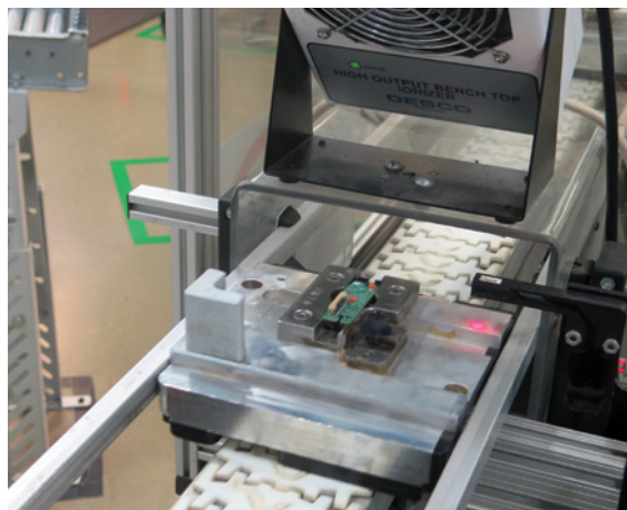
Camera boards pass under ionizing blower during production. Controlling static charges is important in electronics manufacturing due to the impact they can have on device yields. Defects caused by electrostatically-attracted foreign matter can contribute to manufacturing yield losses.
