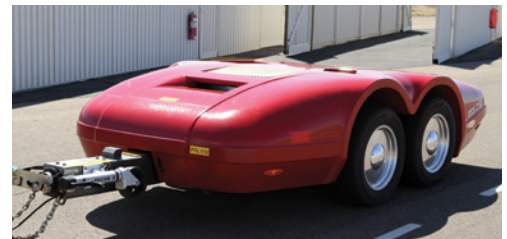
2017 Super Duty prototype with new Taylor RSL-25K dyno sled replicates the Davis Dam climb at Ford's Arizona P.G.
