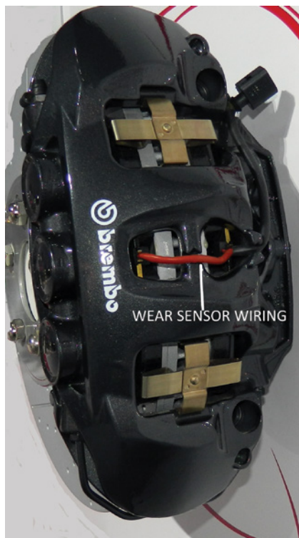
Front caliper is six-piston hydraulic to provide adequate braking for larger cars. It incorporates wear sensors in the brake linings.
