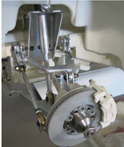
Accurate detail abounds in the CNC machined suspension and brake systems on the 40%-scale Silverado.
