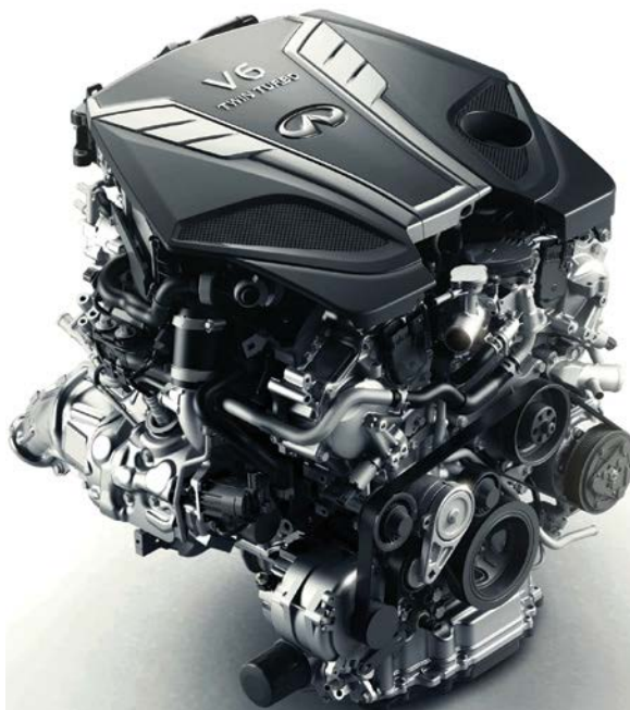
Nissan's all-new 3.0-L VR30DETT—the TT stands for twin turbo—is available in two performance ratings and is thus far an Infiniti-only power unit.
