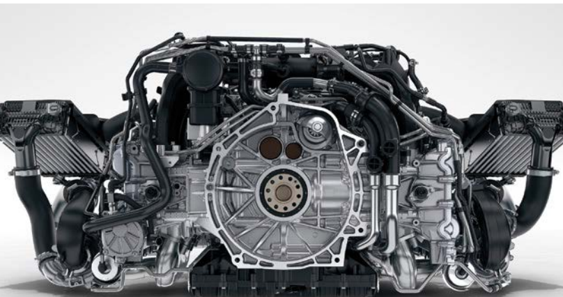
Output-side view of Porsche's all-new 9A2 twin-turbo boxer six. The company's upcoming new turbocharged boxer four-cylinder shares design elements from this unit.
