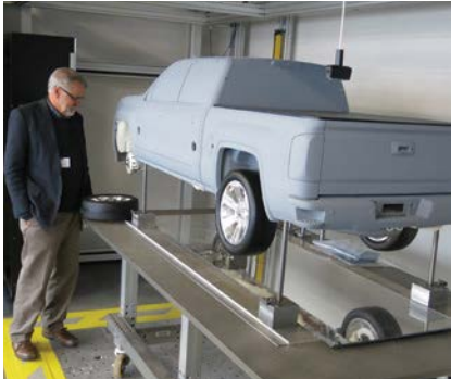
One of GM's new 40%-scale model vehicles, a Chevrolet Silverado, at the new wind tunnel facility in Warren.
