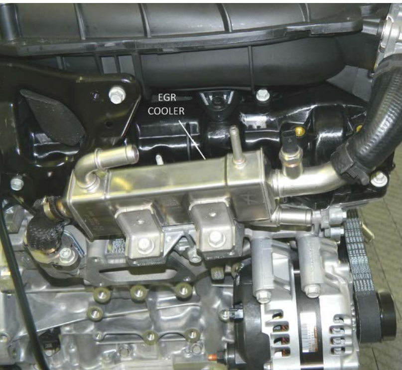
FCA's significantly upgraded 3.6-L Pentastar V6 now includes a liquid-cooled EGR module. (Paul Weissler)
