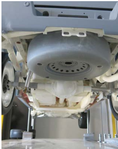
Highly detailed scale model underbody (view from rear of Silverado with spare tire in foreground) created using GM's 3D printing capabilities.
